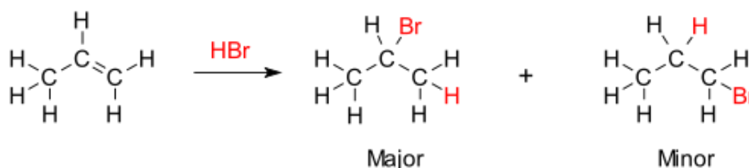
Figure 01: Markovnikov's Rule is illustrated by the reaction of Propene with Hydrobromic Acid
