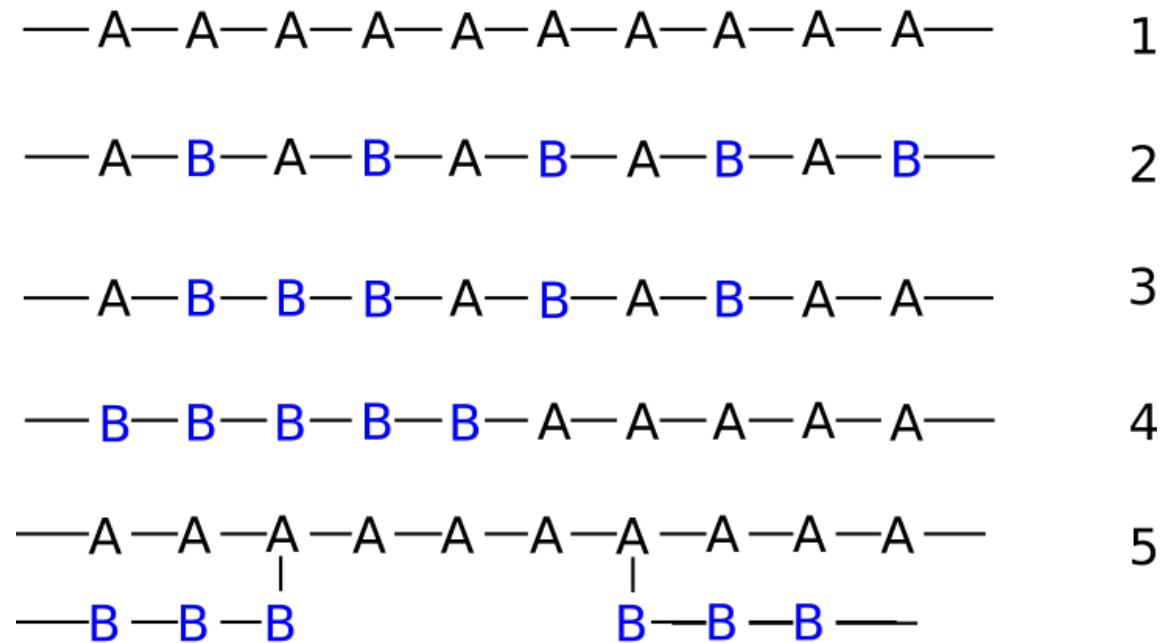
Figure 02: Types of Copolymers (1. Homo-polymer, 2. Alternating polymer, 3. Random copolymer, 4. Block copolymer, 5. Branched copolymers)
